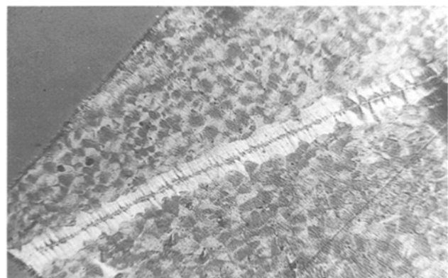
Figure 33 Cylindritic structure containing a large number of \beta -spherulitic segments formed along the weld line.
