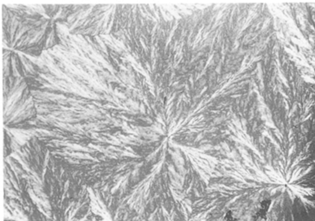
Figure 6 Positive \alpha -spherulite formed in a degraded iPP sample with fibrillar structure resolved at the optical level.
