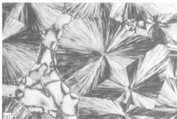
Figure 19 (a) Isothermally crystallized sample consisting of mixed \alpha -spherulites, and its transition into (b) negative and (c) positive spherulites after heat treatment depending on T_F (see text).
